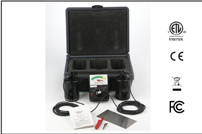
Figure 1. SCS 701 Analog Surface Resistance Megohmmeter Kit.
