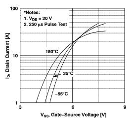
Figure 2. Transfer Characteristics
