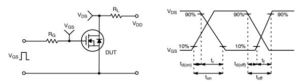
Figure 14. Resistive Switching Test Circuit & Waveforms
