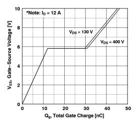
Figure 6. Gate Charge Characteristics
