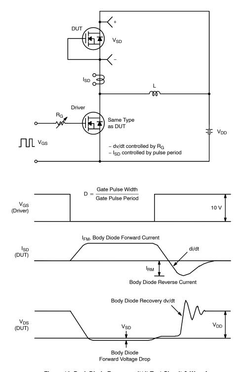
Figure 16. Peak Diode Recovery dt/dt Test Circuit & Waveforms
