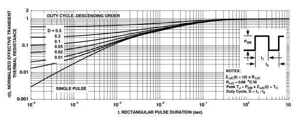
Figure 12. Transient Thermal Response Curve
