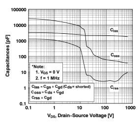
Figure 5. Capacitance Characteristics
