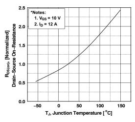
Figure 8. On-Resistance Variant vs. Temperature
