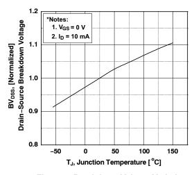
Figure 7. Breakdown Voltage Variation vs. Temperature
