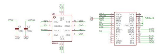
BMA253 shuttle board electrical layout
