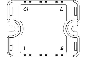
All multiple inputs and outputs must be shorted together 3/4; 5/6; 7/8; 1/2; 9/10
